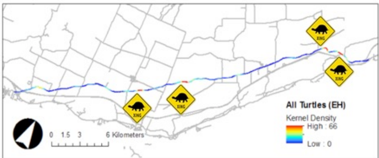
Figure 11. Proposed signage placement for turtle crossings. It is suggested that signs are placed 500m before the hotspots, in both directions.
